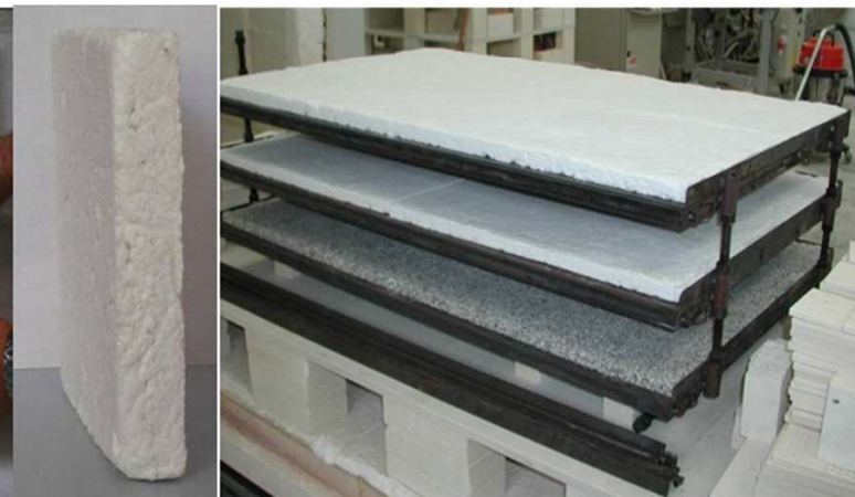
Bio-soluble based light-weight panels ( < 200 \text{ kg}\cdot\text{m}^{-3} ) for thermal and acoustic insulation in naval applications
