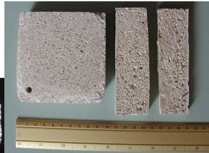
Bio-soluble based light-weight panels ( < 200 \text{ kg}\cdot\text{m}^{-3} ) for thermal and acoustic insulation in naval applications
